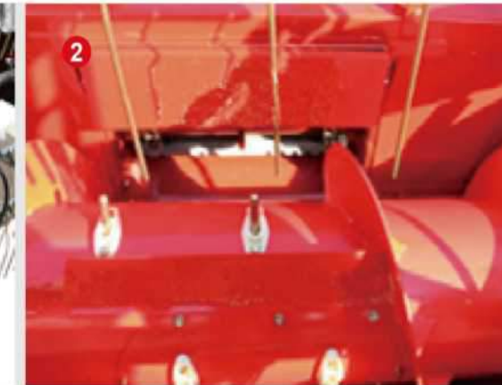
2 No straw twisted ,anti-twister border inner space 20mm between blade and harrow.
