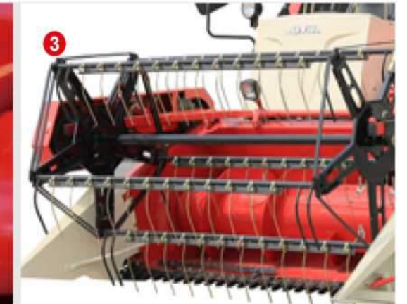
3 Easier for grabbing lodging grain , special design.
