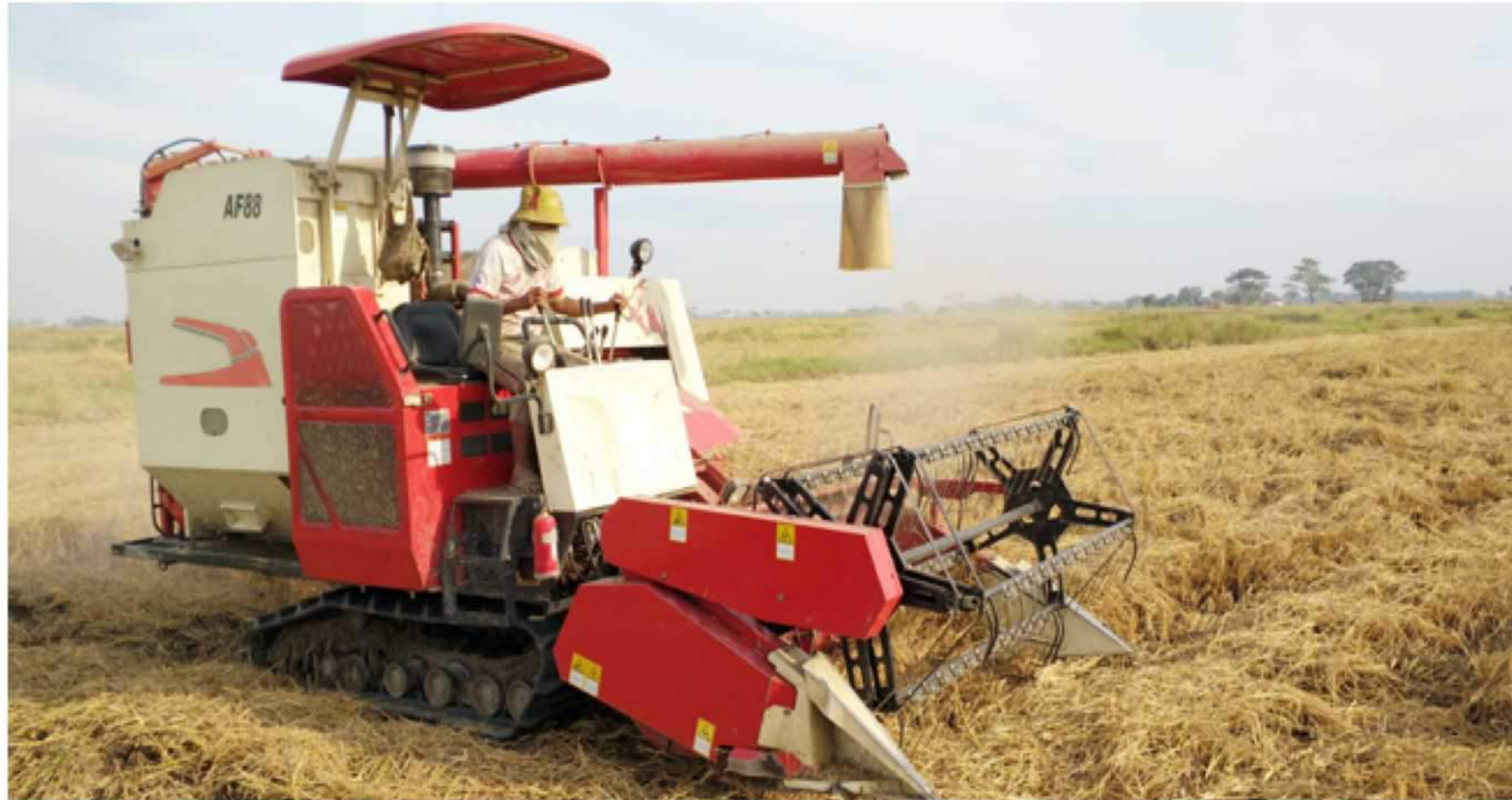
1 Easier for lodging grain , inclined angle header.
