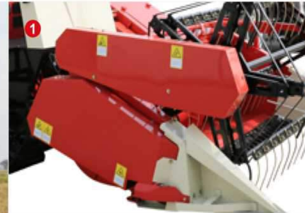
1 Easier for lodging grain , inclined angle header.
